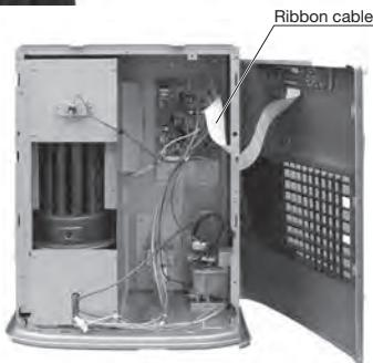
4. Install the WiFi module into the 2 holes on the PCB support.
