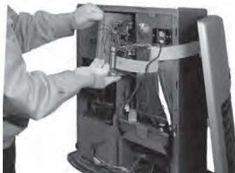
② Insert the lead wire into the WiFi connector of the main circuit board.
