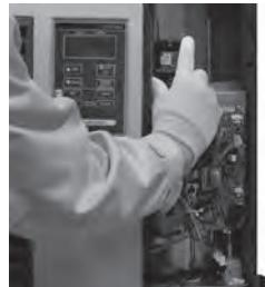
5. Insert the lead wire into the WiFi connector of the main circuit board.
