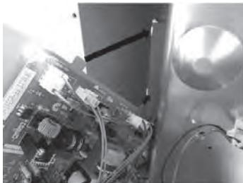
② Tighten the main circuit board bracket with two screws.
