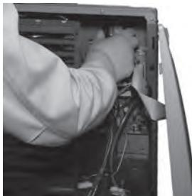
5. Insert the lead wire into the WiFi connector of the main circuit board.
